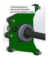
Furthermore, the flange offers also the option to bring pressurized oil to the PTO through an external pipe. In fact, outside on the flange there is a plug G  $\frac{1}{4}$ , which can be removed for the connection of an external pipe.
